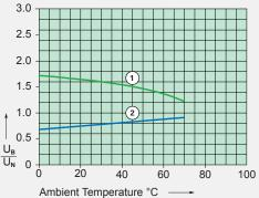
1) Max. excitation voltage with contact load: ≤4A 2) Min. excitation voltage (guaranteed values) without
