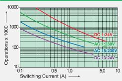
Maximal switching characteristics (DIN EN60947-5-1,
