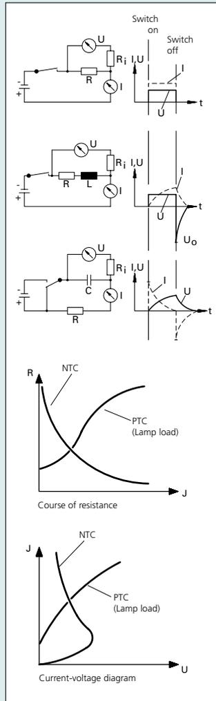
Posistor lamp load: High inrush current occurs when posistors (iron-hydrogen resistor, heating coils, e.g. made of tungsten) of electrode tubes and resistance furnaces.
